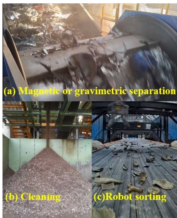
Figure 3. Recycling considering different steps of (a) magnetic or gravimetric separation, alongside (b) cleaning and (c) Robot sorting to enhance scrap metal quality by reducing tramp elements.
